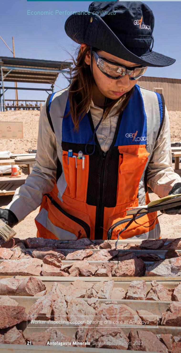
Worker inspecting copper-bearing drill core at Antucoya
